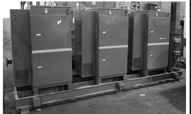
Bauer #AT75-E3, 25 HP Rotary Screw Air Compressor
